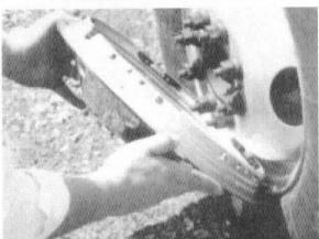
Set the wheel cover in position at the base of the wheel and tip it up on to the wheel making certain the valve stem cut out is properly aligned with the valve stem.
